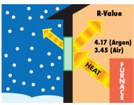
Note: All comparisons are based on windows containing 3/4" insulating units; two 1/8" (3mm) glass lites and a 1/2" (12mm) air- or argon-filled space for the standard clear insulating glass and the Solarban® 70XL insulating glass. Actual glass performance may differ slightly due to glass thickness, gas fill and glass to frame ratio.
