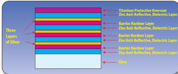
On the glass facing the outside of your home, **UltraFlect** places a coating that is State of the Art in reflecting damaging UltraViolet and heat-carrying infrared rays from the sun
