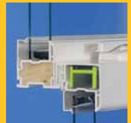
Full Continuous Meeting Rail Interlock With Dual Fin Seal Weather Stripping
