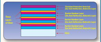
On the glass facing the outside of your home, **UltraFlect** places a coating that is State of the Art in reflecting damaging UltraViolet and heat-carrying infrared rays from the sun
